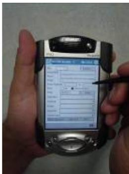
They are small, hand held devices that operate on the pocket PC system. The CCTV header information and survey observations can be made at the time of survey.
