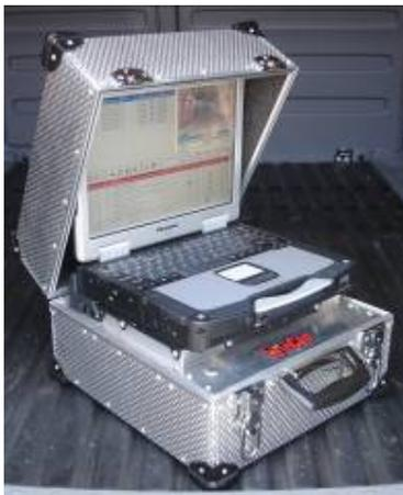
This system comprises a Panasonic Toughbook CF-30 and purpose made case. The Panasonic laptop can be removed from the docking-station. The system is portable (12.5Kg) and runs from its own battery supply so there is no need for generators etc. The metal case houses the WinCan digital MPEG recorder.
